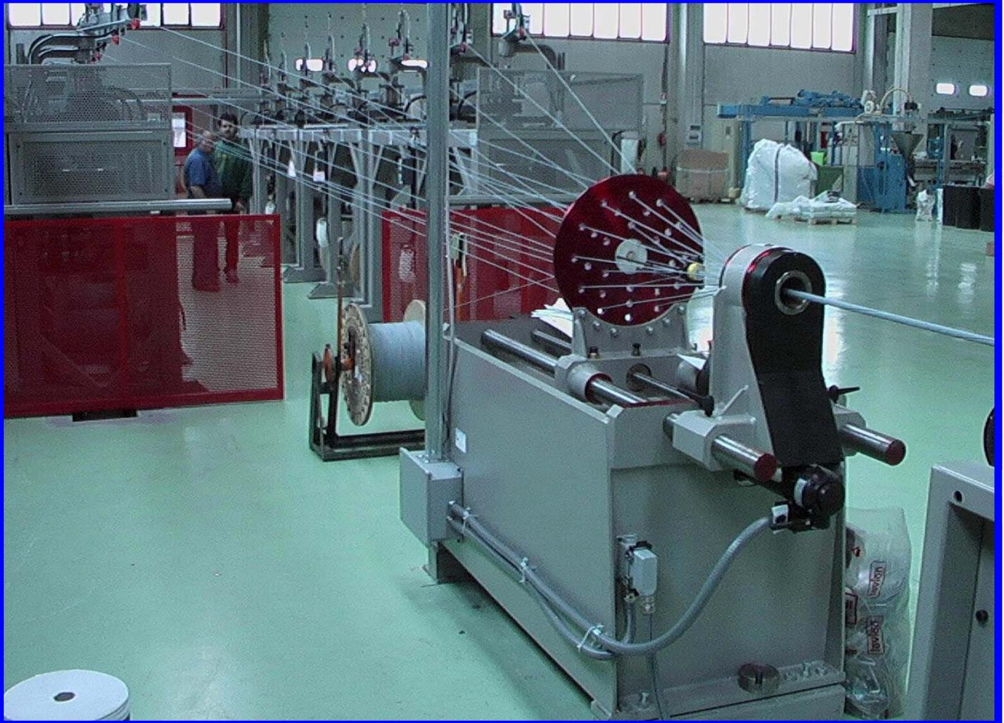
LINEA DI RIUNIONE MONOTORSIONE PER CAVI SPECIALI, MICROCOASSIALI, MULTI L.A.N. E CAVI A FIBRE OTTICHE. LA LINEA E' ATTEZZATA CON SVOLGITORI A DETORSIONE COMPLETA 100% O ,A SCELTA ,LA DETORSIONE PUO' ESSERE PROGRAMMATA CON PERCENTUALI PIU' BASSE. LA LINEA E' OVVIAMENTE PREDISPOSTA PER L'APPLICAZIONE DI PIU' NASTRI LONGITUDINALI OLTRE AD AVERE LA POSSIBILITA' DI NASTRARE AD ELICA CHIUSA O CONTROVERSA .LE BOBINE DI RACCOLTA SARANNO 1250 1000 E 800 DIN.
